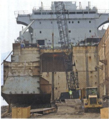
Ships are pulled ashore by giant cables and 'sliced like a salami.'
